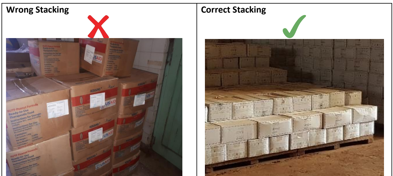
Figure 8.4: Correct and wrong stacking methods
